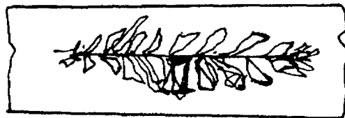
Figure 1.41: Piping in weld.
