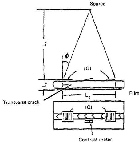
Figure 10.7 Radiographic arrangement for determining the angle of radiation relative to transverse crack
