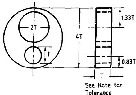
Design for Penetrator Thickness of 0.180 in. and Over
