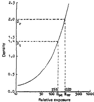
Figure 6.18 Characteristic curve for a typical direct type film.
