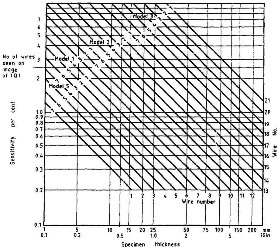
Method of use. Read off the number of wires visible on the appropriate model of I.Q.I. against the specimen thickness.
