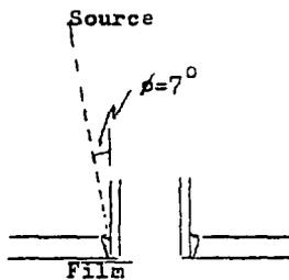
Figure 8.7 Radiography of nozzle welds.
