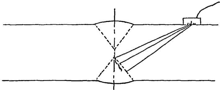
Figure 1.27 Illustration of ragged weld crack
