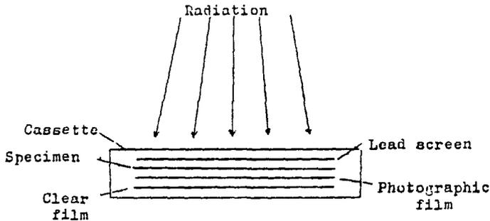
Figure 8.20 Arrangement for electron transmission radiography.
