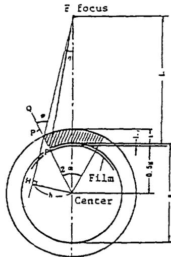
Figure 8.6 Internal film technique
