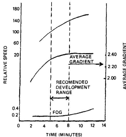
Figure 4.12 Dependence of the characteristics of a typical radiographic film on the development time
