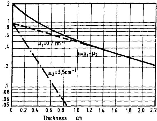
Figure 2.17. Attenuation of a radiation beam composed of two different energies
