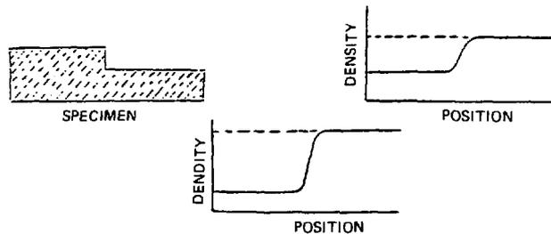
Figure 6.13 Illustration of radiographic contrast.
