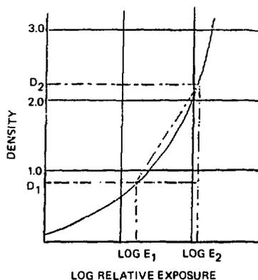
Figure 4.10 Measurement of slope (contrast) as an average between two densities.
