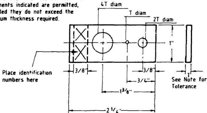
Design for Penetrator Thickness from 0.060 in. to and Including 0.160 in. Made in 0.010 in. Increments.
