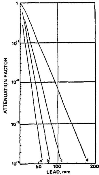
Figure 12.9 Absorption of gamma rays in lead : broad beam conditions
