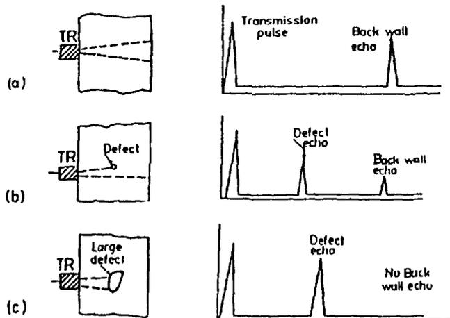
Figure 1.24 Principle of pulse echo method of ultrasonic testing. (a) defect free specimen (b) specimen with small defect (c) specimen with large defect.
