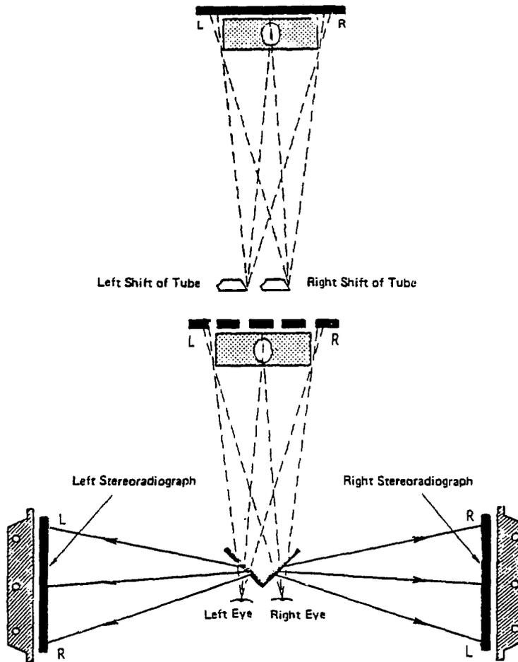
Figure 8.16 Schematic diagrams showing the methods of making and viewing stereo-radiographs.
