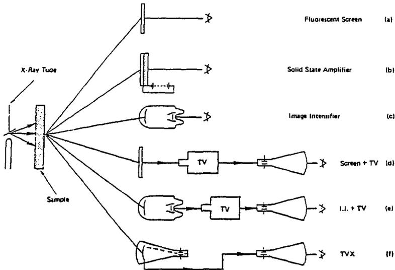
Figure 4.19 Summary of different fluoroscopic arrangements.
