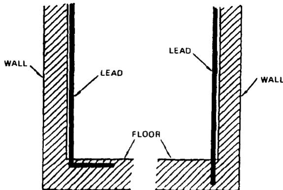
Figure 12.5 Method of lead lining the floor
