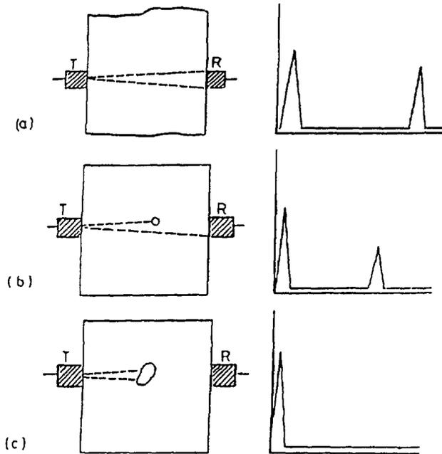
Figure 1.23 (a) Defect free specimen, (b) Specimen with a small defect, (c) Specimen with a large defect.
