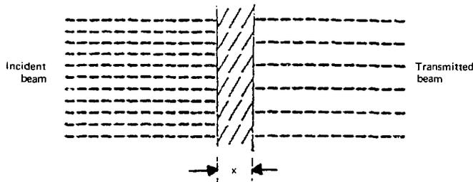
Figure 2.10. Absorption of radiation.
