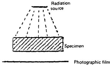
Figure 6.1 Source, specimen and film arrangement to obtain a radiograph.
