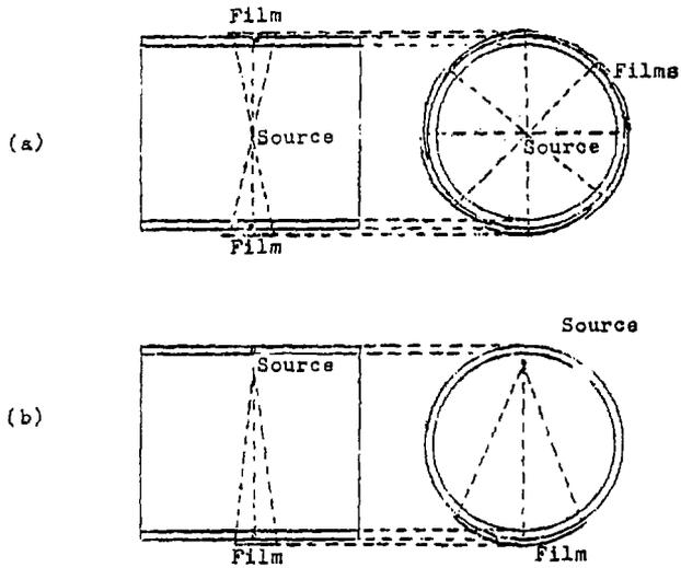
Figure 8.3. Film outside, source inside arrangement.
