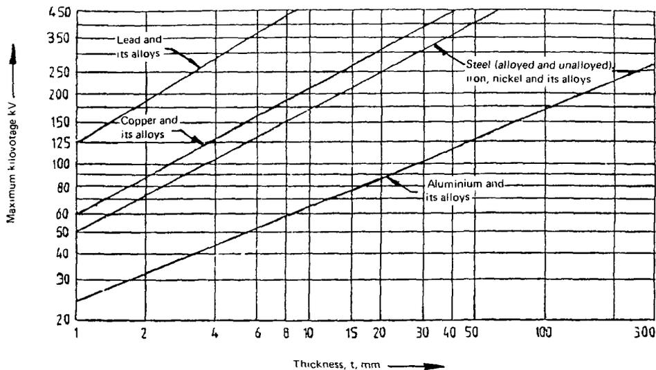
Figure 10.8 Maximum kilovoltage for X-rays up to 450KV for different materials for classes A and B in terms of material thickness.
