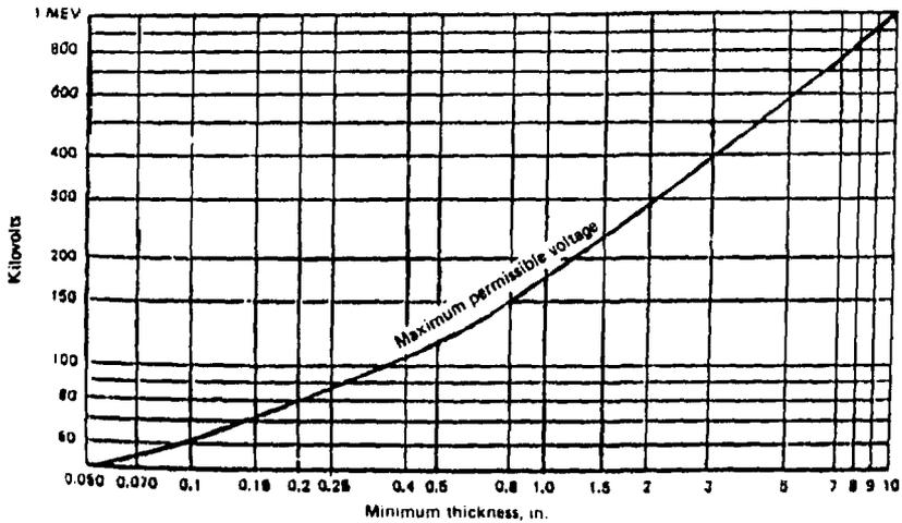
Figure 10.10(c) Max.voltage permissibe for Al and Al alloys.
