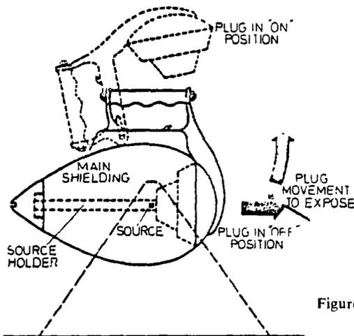
Figure 3.10 Removable plug type gamma projector
