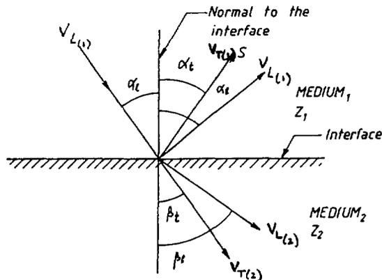
$v_{L(1)}$  and  $v_{L(2)}$  = velocities of longitudinal waves in material 1 and 2 respectively.
