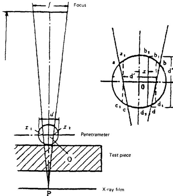
Figure 7.3 Absorption of X-rays by wire of penetrometer
