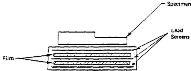
Figure 8.17 Double film technique
