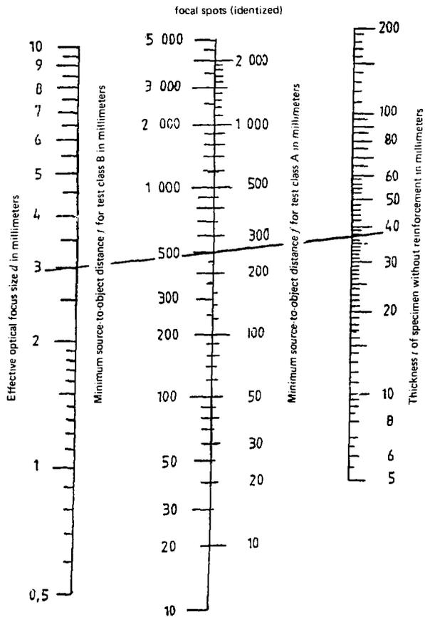
Figure 10.3 Nomogram for calculation of  $f$
