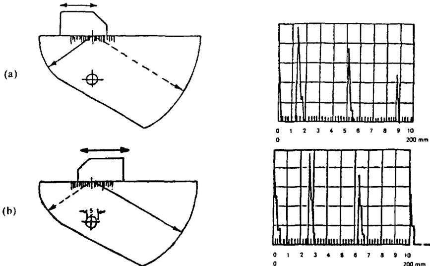
Figure 1.20 V2 test block (a) with the probe index at the zero point and directed to the 25mm radius, (b) with the probe index at the zero point and directed to the 50mm radius.
