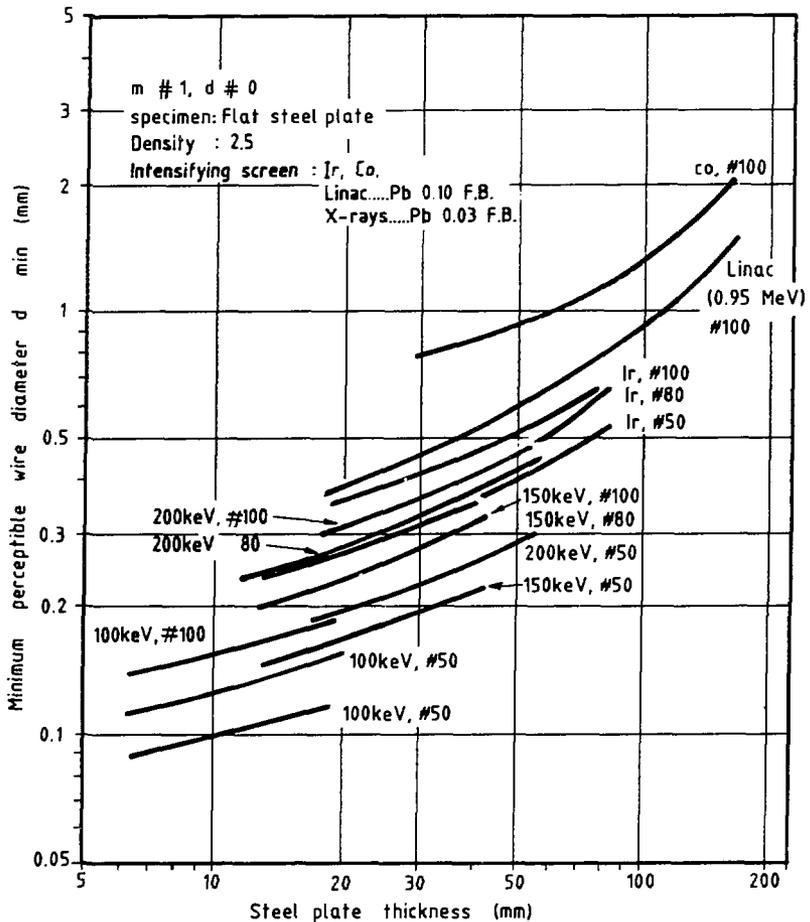
Figure 7.17 Relationship between the types of radiation source, film and screen and the minimum perceptible wire diameter
