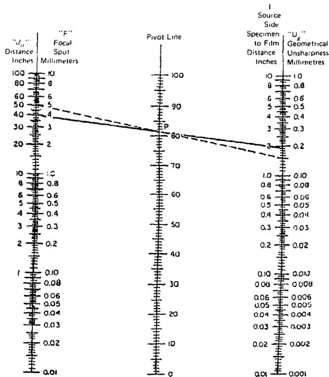
Figure 10.6 Nomogram for determining geometric unsharpness.
