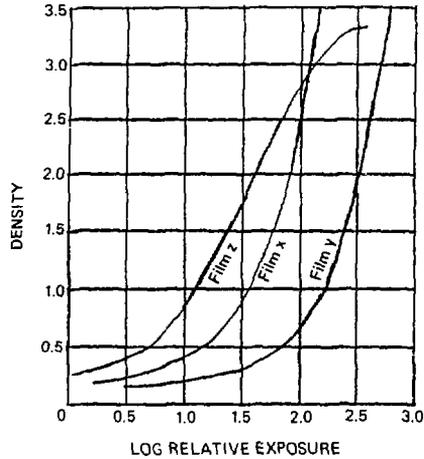
Figure 4.5 Characteristic curves of three typical industrial radiographic film
