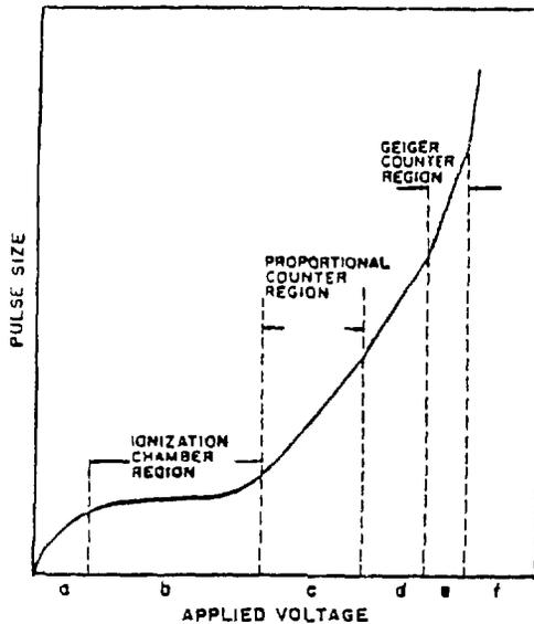
Figure 2.19 Pulse size as a function of applied voltage in gaseous ionisation chamber.
