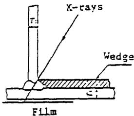
Figure 8.9 Thickness compensating wedge
