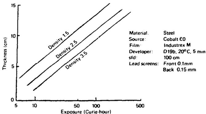
Figure 6.21 A typical gamma ray exposure chart.
