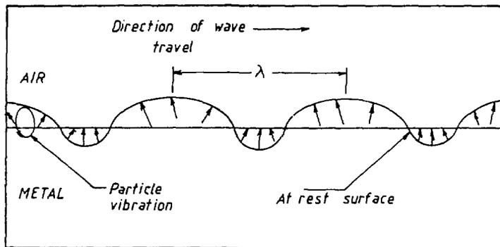
Figure 1.13 Diagram of surface wave propagating at the surface of a metal along a metal - air interface.
