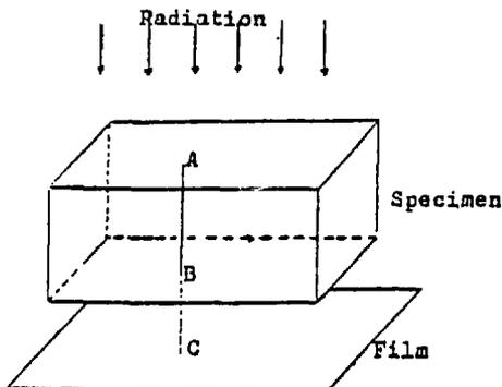
Figure 8.11 Two dimensional shadow formation of a defect.
