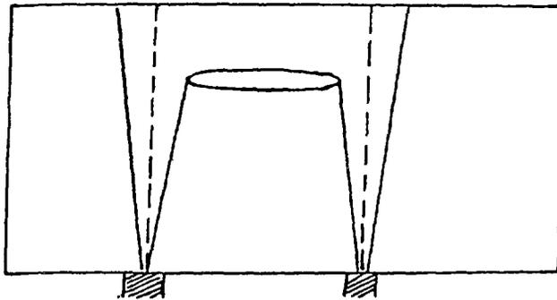
Figure 1.26 20 dB method of defect sizing
