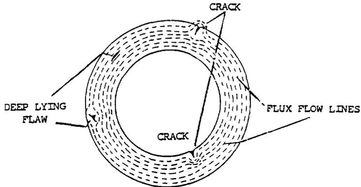
Figure 1.2(b): The effect of defects on the flux flow in a magnetised ring.
