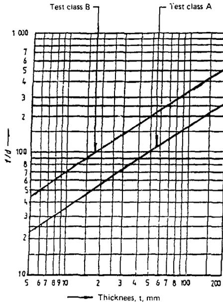
Figure 10.1 Required minimum values of ratio  $f/d$  in terms of thickness  $t$
