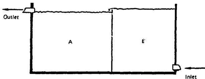
Figure 5.3 Cascade washing tanks
