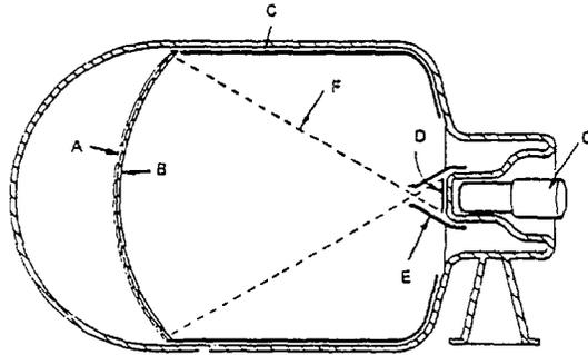
Figure 4.16 Norelco industrial image intensifier (A) Fluorescent screen (B) Photocathode (C) Conductive coating (D) Viewing screen (E) Anode (F) Electron paths (G) Optical system
