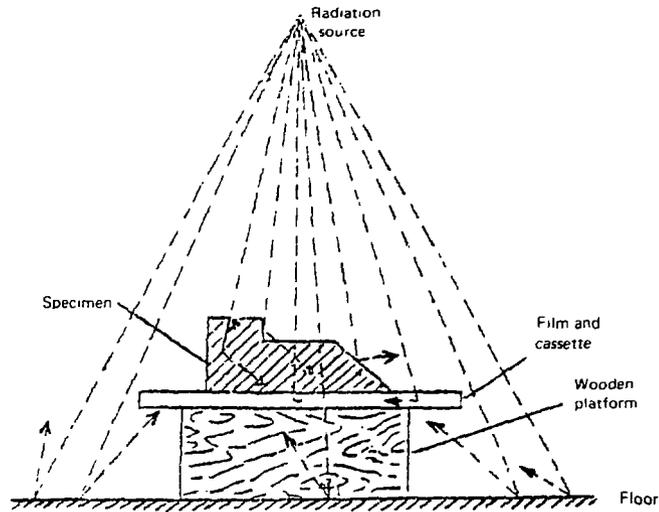
Figure 6.16 Sketch showing sources of scattered radiation while taking radiograph of an object.
