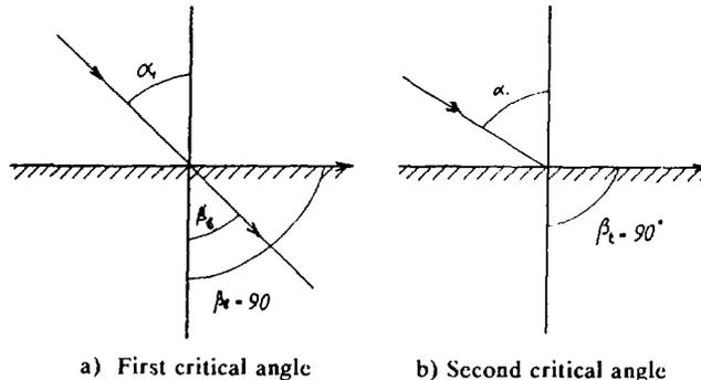
Figure 1.15 First and Second Critical Angles
