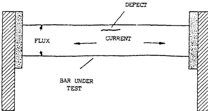
Figure 1.3 : Flux flow in a bar carrying current.
