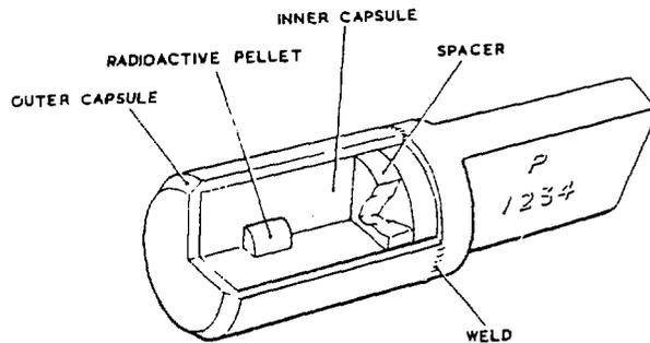
Figure 3.9 Cut away of a typical radiography source
