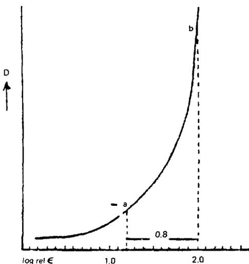
Figure 6.22 Exposure range calculation.
