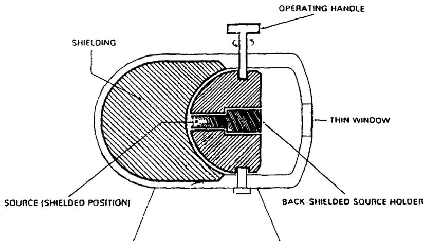
Figure 3.11 Rotating shutter type exposure container
