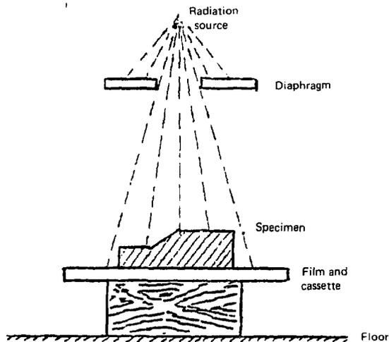
Figure 6.17 Sketch elaborating the use of a diaphragm.
