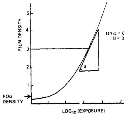
Figure 4.6 Typical characteristic curve for 'direct' x-ray film.
