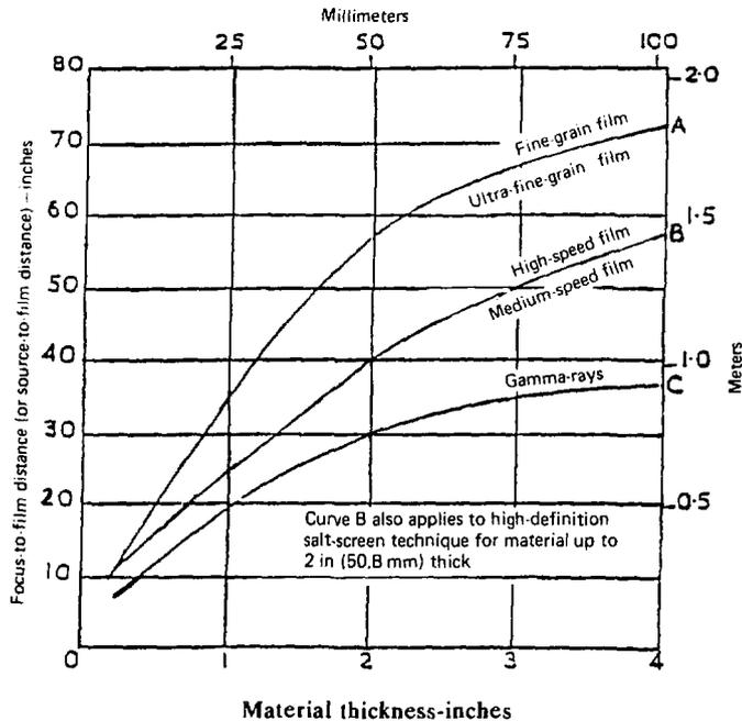
Minimum values of focus-to-film distance (or source-to-film distance) Calculated for 7mm focal spot (Curves A and B) 4mm source (Curve C)
