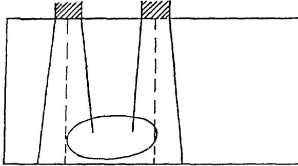
Figure 1.25 Defect sizing using the 6 dB drop method
