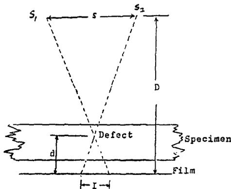
Figure 8.13 Tube shift method.
