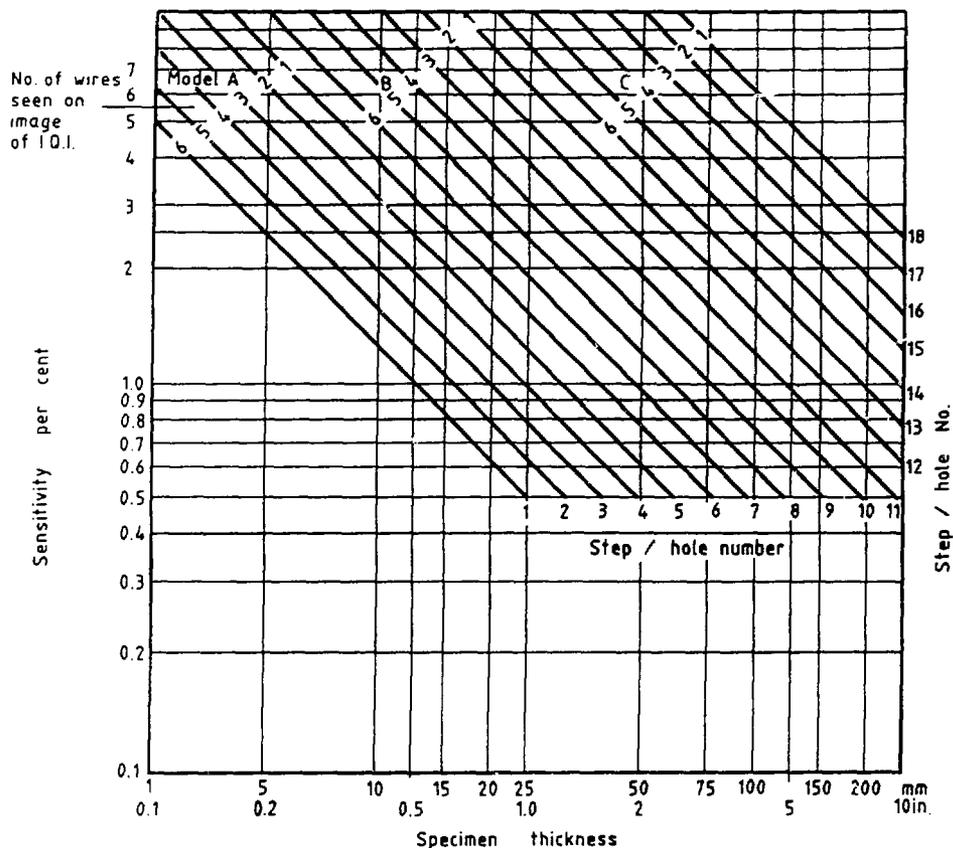
Method of use. Read off the number of steps on the image of the I.Q.I. in which holes are visible on the appropriate model, against the specimen thickness.
