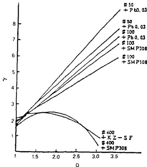
Figure 7.2 Relationship between density and film contrast for different combinations of X-ray films and intensifying screens.
