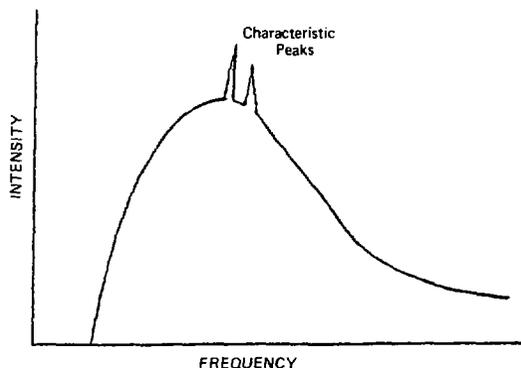
Figure 2.2 Characteristic x-ray spectrum
