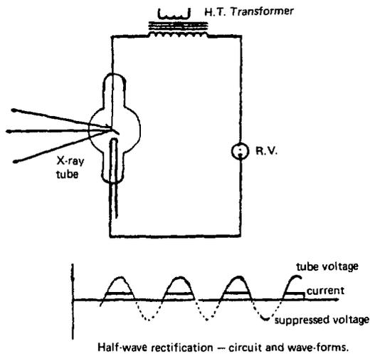
Figure 3.4 Single valve circuit
