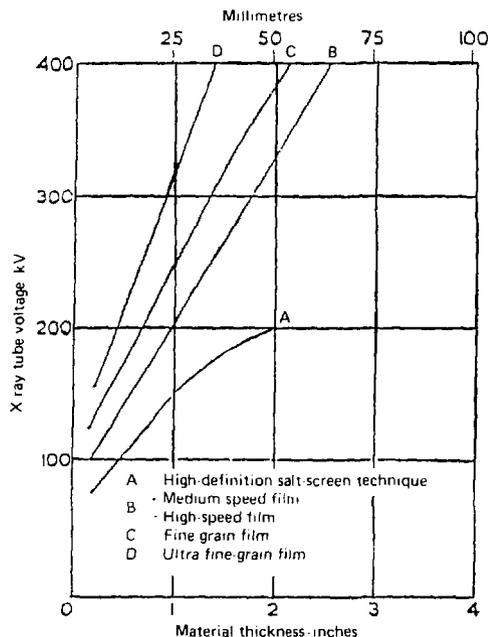
Figure 10.9 Maximum X-ray tube voltage according to B.S.2600
