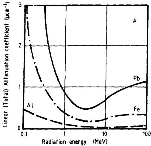
Figure 2.16 Variation of attenuation coefficients of  $\mu$ . Al, Pb and Fe with radiation energy
