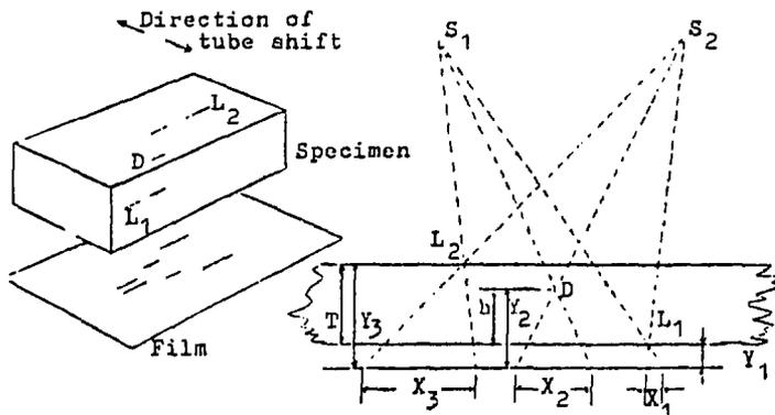
Figure 8.14 Lead marker method.
