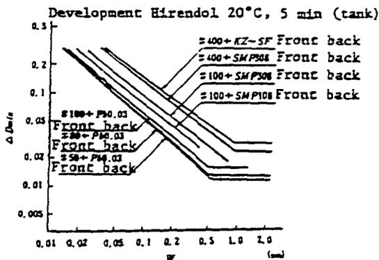
Figure 7.13 Relationship between wire image width of X-ray films and intensifying screens and  $\Delta D_{\min}$  for different combinations.
