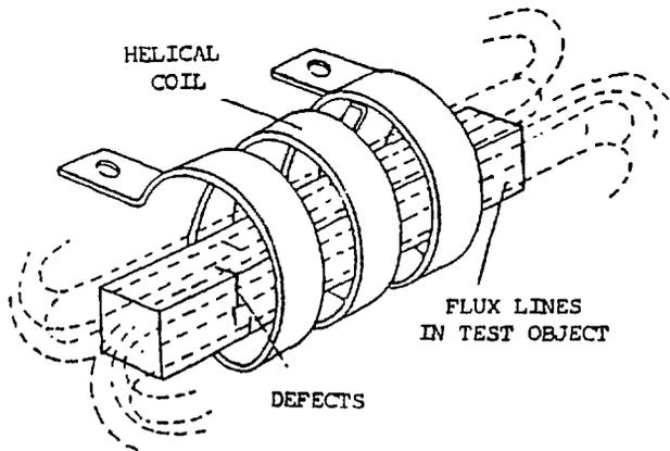
Figure 1.7 : Helical Coil
