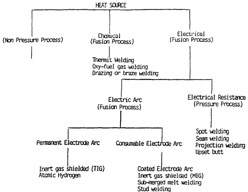
Figure 1.36 : Different processes of welding
