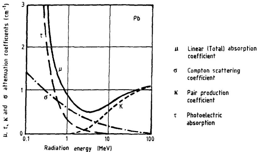
Figure 2.15 Energy dependence of attenuation coefficient and its various components
