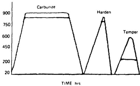
Figure 1.38 Typical heat treatment cycle for carburizing
