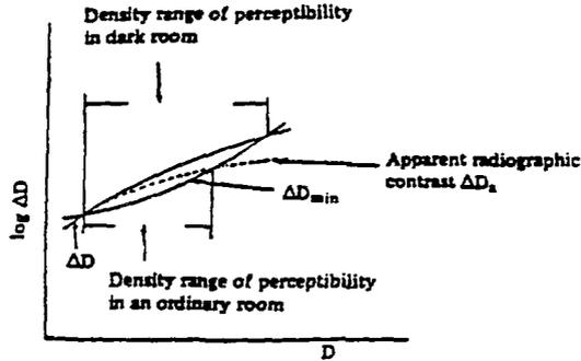
Figure 7.15 Relationship between density,  $\Delta D$  and  $\Delta D_{min}$  (influence of room brightness)
