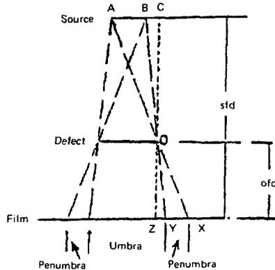
Figure 6.3 Formation of shadow of a defect.
