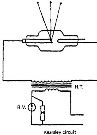
Figure 3.3. Self rectifying circuit
