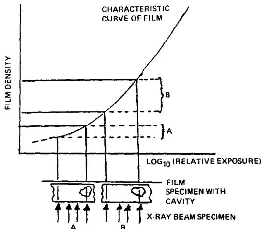
Figure 4.7 Diagram to illustrate the effect of using a higher working density on a radiographic film. A is the density difference in the image of the cavity after a short exposure. B is the density difference in the image of the cavity after a longer exposure.
