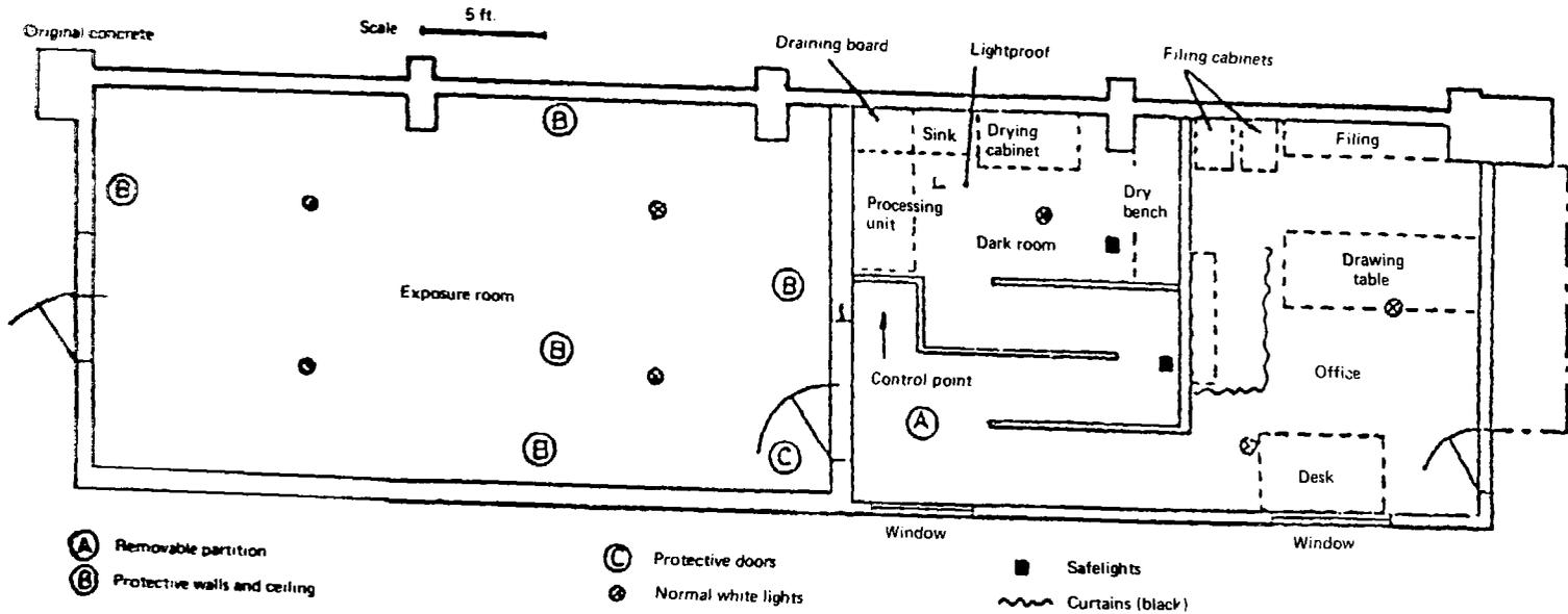
Figure 12.4 Floor plan of radiographic section
