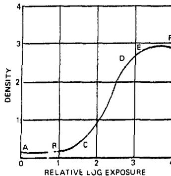
Figure 4.3 Characteristic curve of a typical salt-screen X-ray film.
