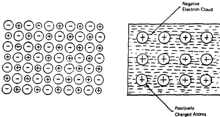
Figure: 1.31 Schematic illustration of a metallic bond
