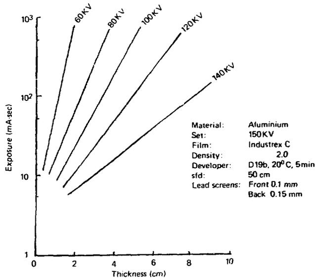
Figure 6.19 A typical exposure chart.
