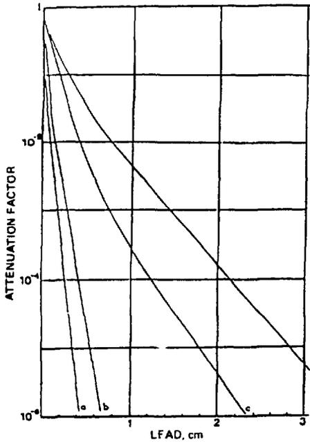
Figure 12.8 Attenuation of X-rays in lead: broad beam conditions.
