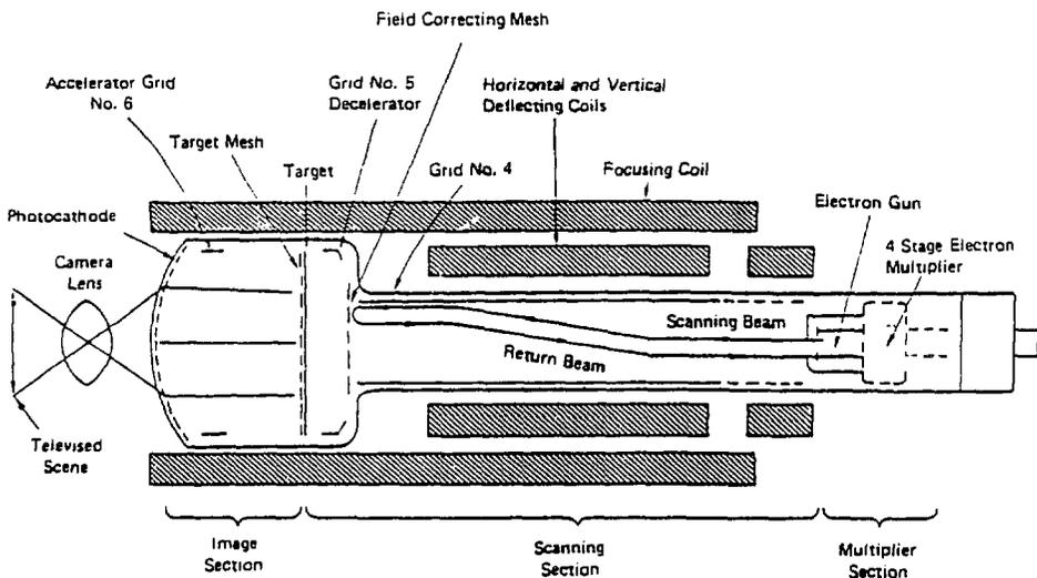
Figure 4.18 Image orthicon tube
