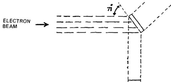
Figure 3.2 Actual Vs effective focal spot size
