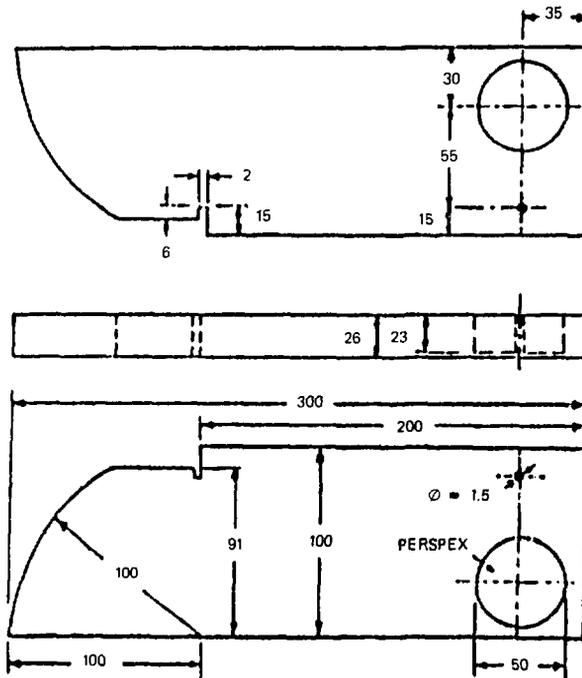
Figure 1.19 I.I.W test block
