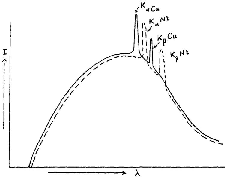
Figure 2.3 Characteristic X-ray spectra for Cu and Ni
