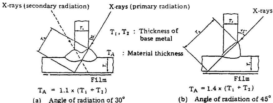
Figure 8.8 Direction of radiation of X-rays and material thickness for T - welds.
