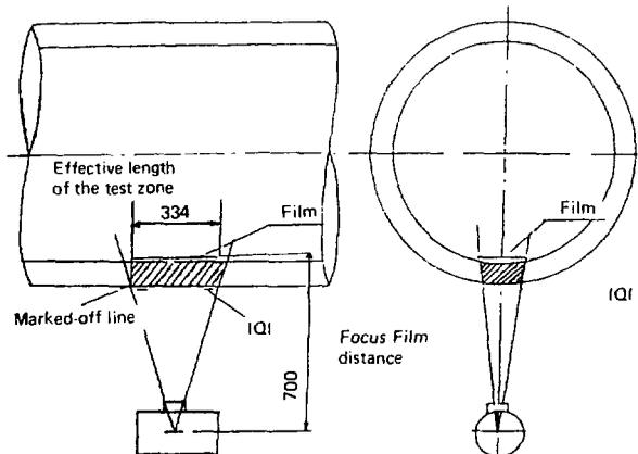
Figure 10.17 Test arrangement for circumferential joints.
