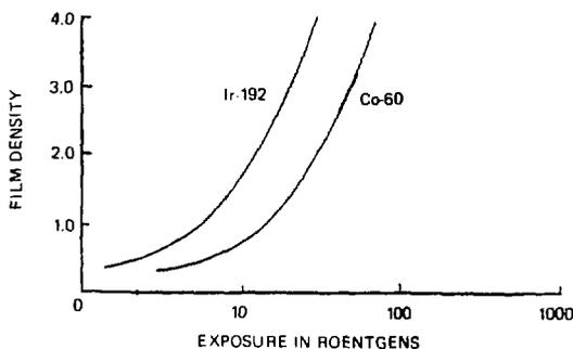
Figure 4.4 Effect of change of radiation quality on the characteristic curve of structurix D2 film.
