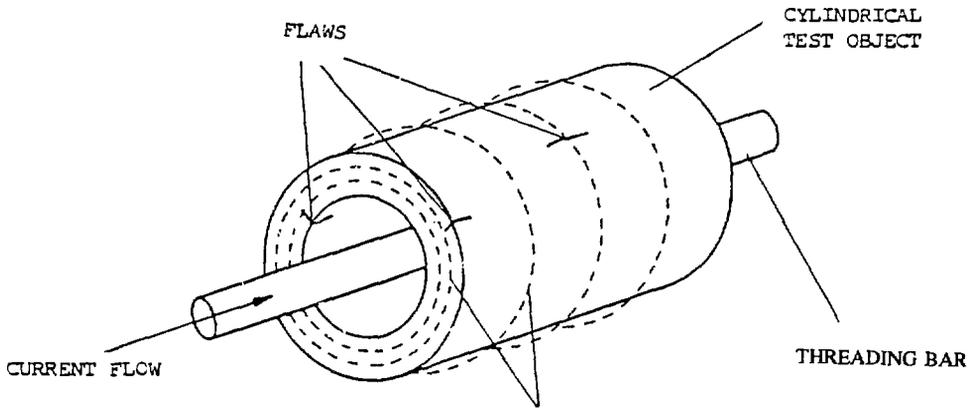
Flux flow in cylindrical specimens using threading bar.
