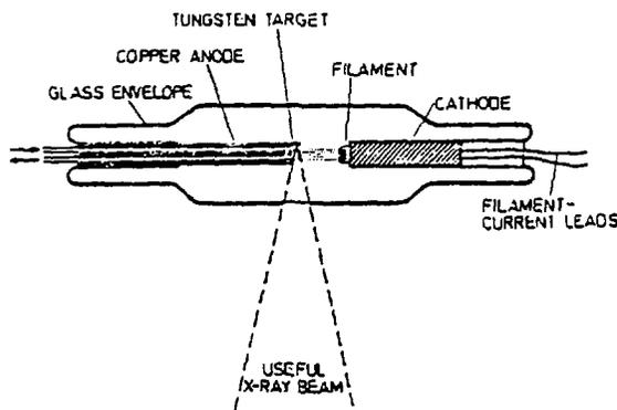
Figure 3.1 A typical X-ray tube
