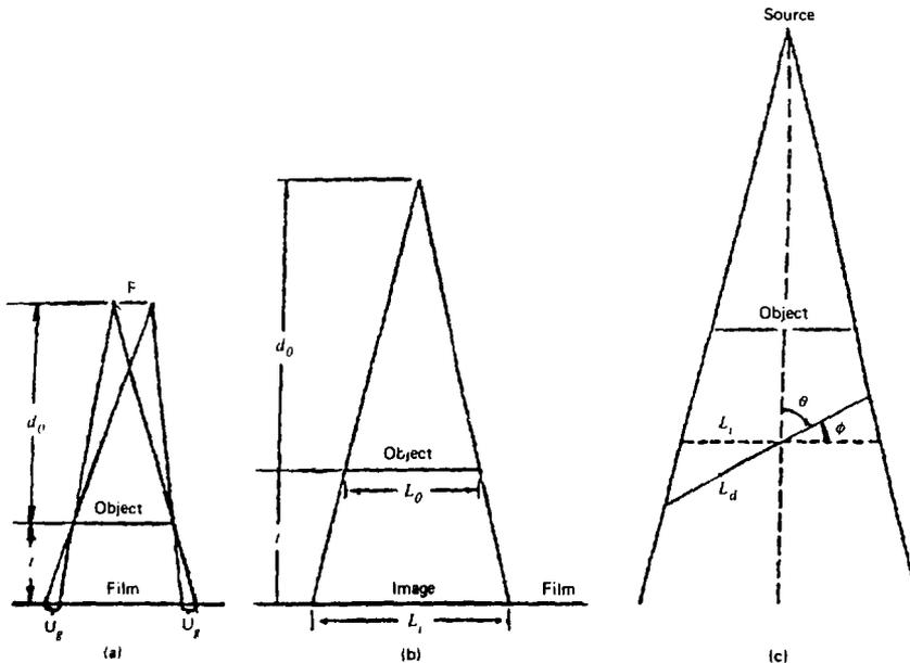
(a) Geometric Unsharpness,  $U_g$  (b) Radiographic Enlargement (c) Radiographic Distortion
