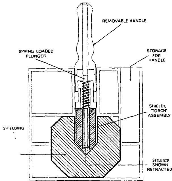
Figure 3.12 Torch type exposure container
