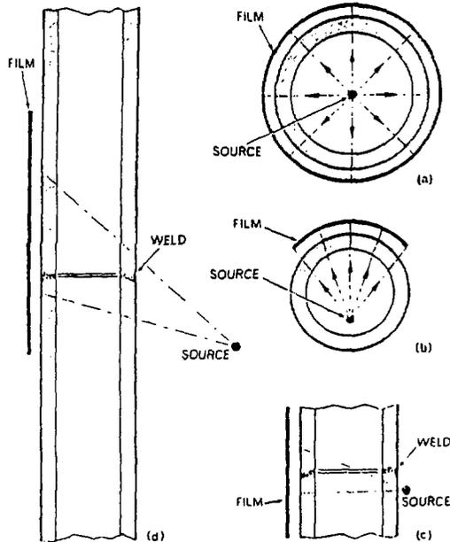
Figure 3.14 Techniques in gamma radiography of pipe welds
