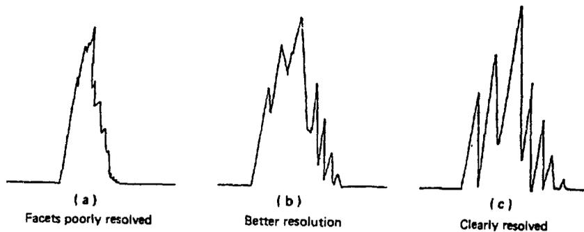
Figure 1.28 Response from weld crack
