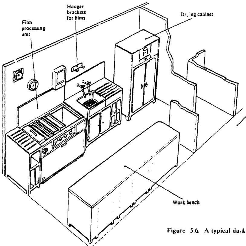
Figure 5.6 A typical darkroom layout.
