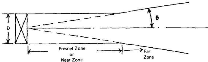
Figure 1.18 Ultrasonic beam from a transducer showing the near and far fields(simplified)
