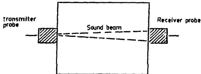
Figure 1.22 Position of transmitter probe and receiver probe in the direct transmission method of ultrasonic testing.
