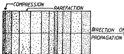
Figure 1.11 Longitudinal wave consisting of alternate rarefactions and compressions along the direction of propagation.
