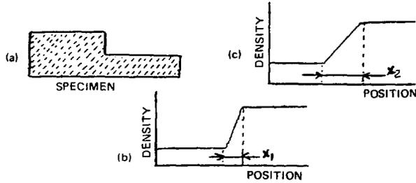
Figure 6.15. Illustration of radiographic definition.
