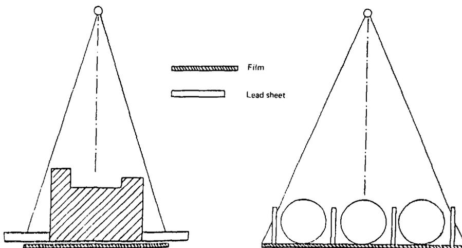
Figure 10.11 Methods of reducing the effect of scattered radiation
