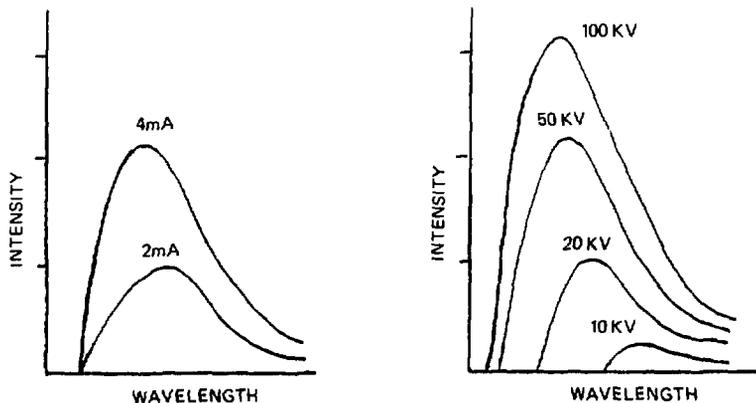
Figure 3.8 Effect of mA and KV on X-ray output
