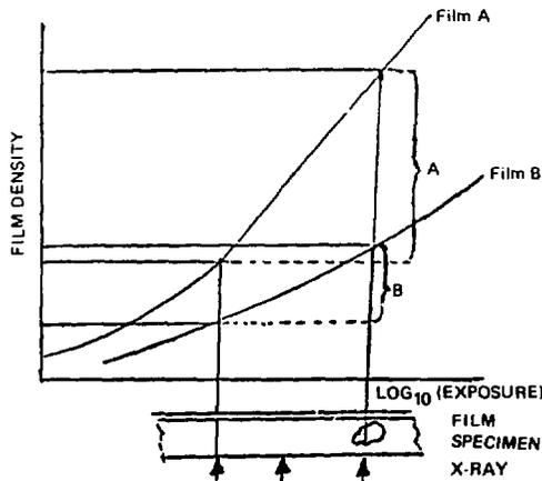
Figure 4.8 Diagram to illustrate the use of a greater film gradient at the working density on radiographic film. A is the density difference in the image on film A. B is the density difference in the image on film B.
