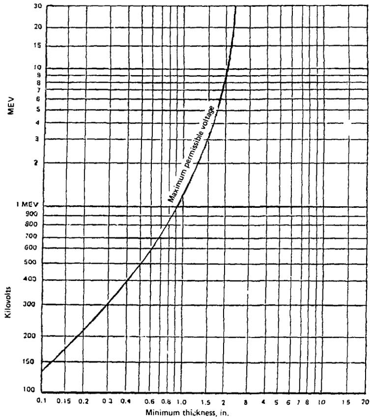
Figure 10.10(b) Max.voltage for alloys of copper and/or high nickel.
