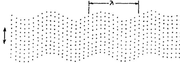
Figure 1.12 Schematic representation of a transverse wave.
