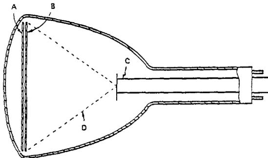
Figure 4.17 Photoconductive X-ray pick-up tube employed by Vidicon Television Systems. (A) X-ray sensitive plate (B) Screen grid (C) Electron gun (D) Electron beam
