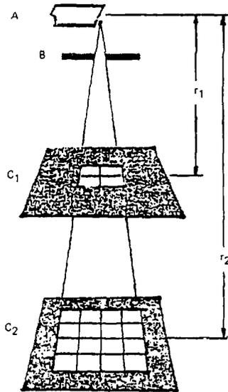
Figure 2.5 Schematic diagram illustrating the inverse square law
