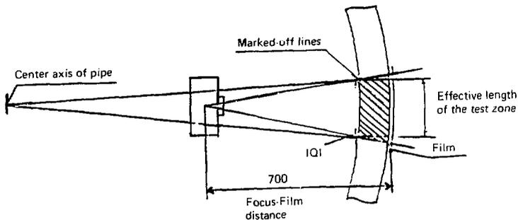
Figure 10.16 Test arrangement for longitudinal joints.
