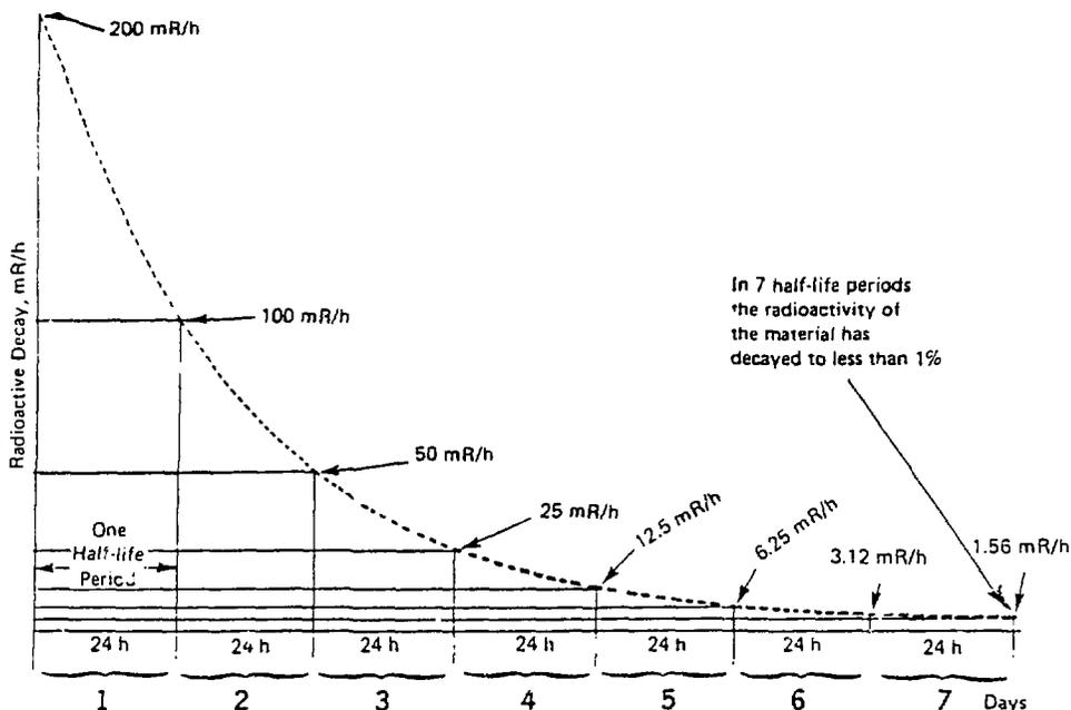
Figure 2.6 Decay of radioactive material with a 24 h half-life
