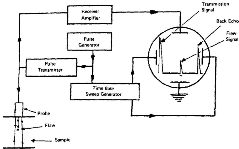
Figure 1.16 A typical ultrasonic test unit
