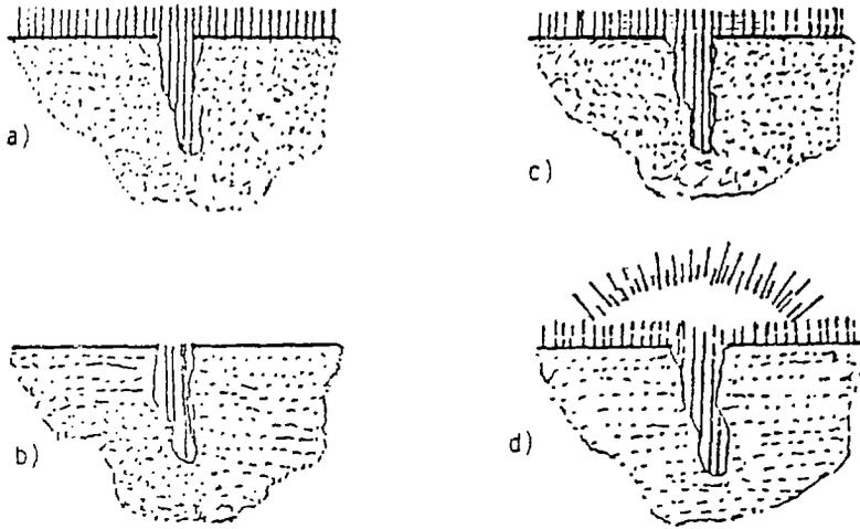
Figure 1.1 Four stages of liquid penetrant process
