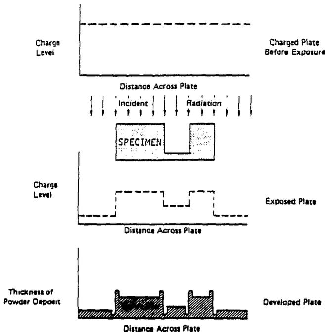
Figure 4.20 Diagrammatic representation of xeroradiography
