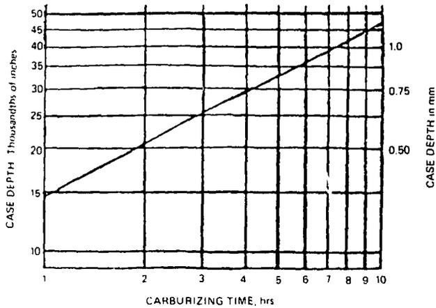
Figure 1.37 Typical carburizing case depth - time relationship.
