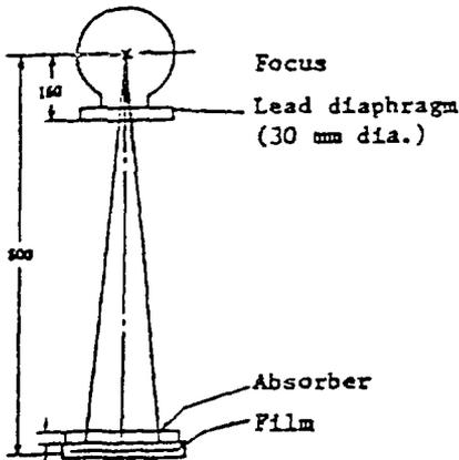
Figure 7.5 Radiographic arrangement
