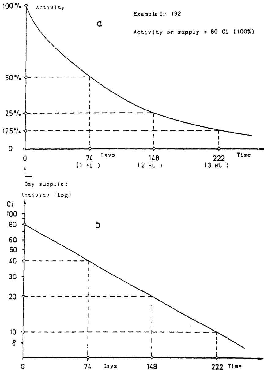
Figure 2.7 : Decay curves of radioactive source, eg. Ir-192 (a) Fall in activity over time. (b) Fall in activity using logarithmic activity scale.
