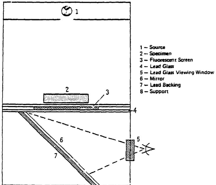
Figure 4.14 Fluoroscopic arrangement with mirror
