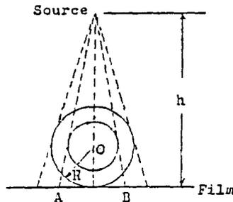
Figure 8.19 Wall thickness measurement of small diameter pipe.
