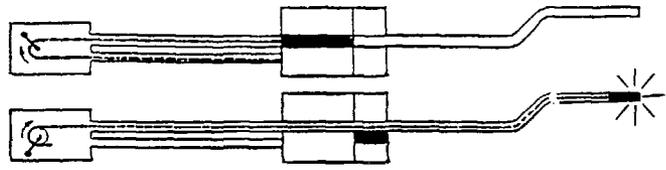
Figure 3.13 Principle of remote control gamma projector
