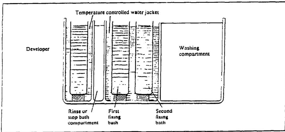
Figure 5.4 Manual processing tanks
