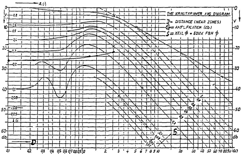
Figure 1.29 Universal DGS diagram.
