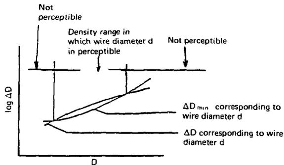
Figure 7.1 Relationship between density,  $\Delta D$  and  $\Delta D_{min}$
