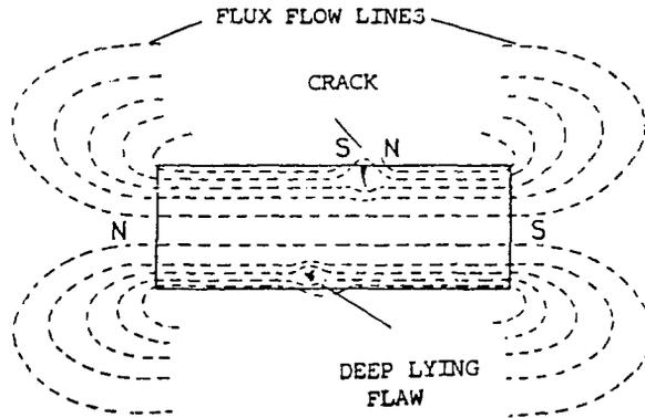
Figure 1.2(a): The effect of defects on the flux flow
