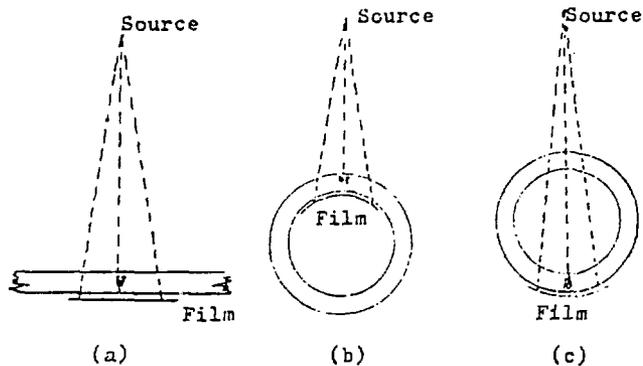
Figure 8.1 Radiography of seam welds.
