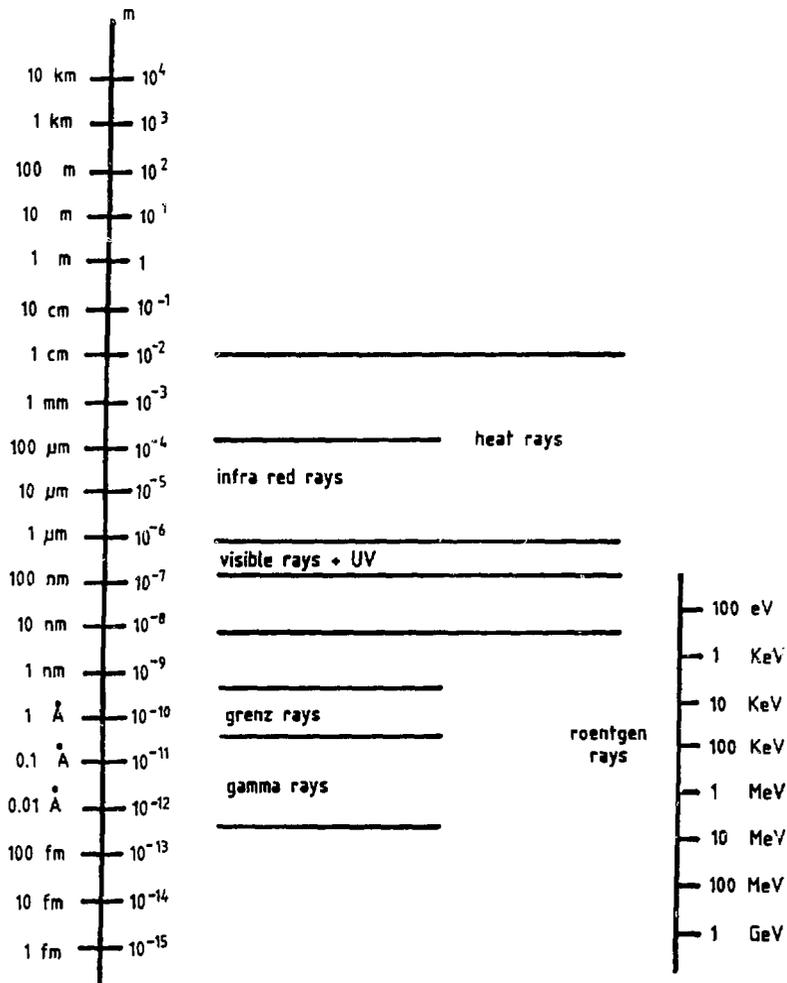
Figure 2.1 Electromagnetic radiation spectra
