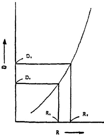
Figure 7.7 X-ray film dose characteristic curve
