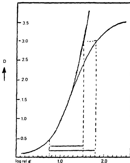
Figure 6.23. Exposure range for two different X-ray films.
