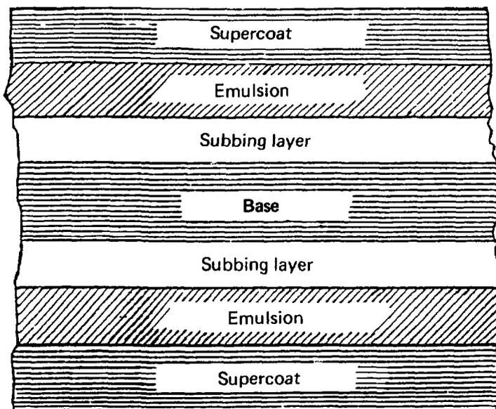
Figure 4.1 Construction of radiographic films.
