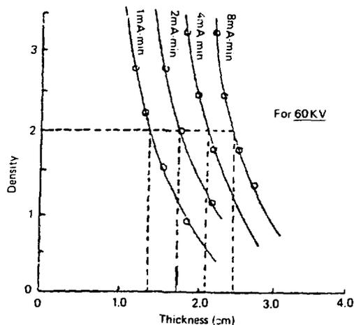
Figure 6.20 Thickness-density curves for various exposures.
