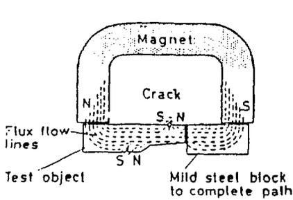
Figure 1.5 : Use of permanent magnet.
