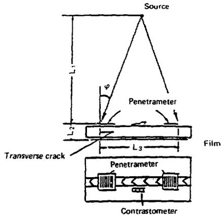
Figure 6.25 Radiographic arrangement for determining angle of radiation relative to transverse crack
