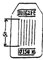
Figure 6.5. Design of DIN type image quality indicators.
