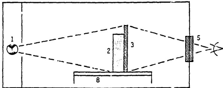
Figure 4.15 Fluoroscopic arrangement without mirror
