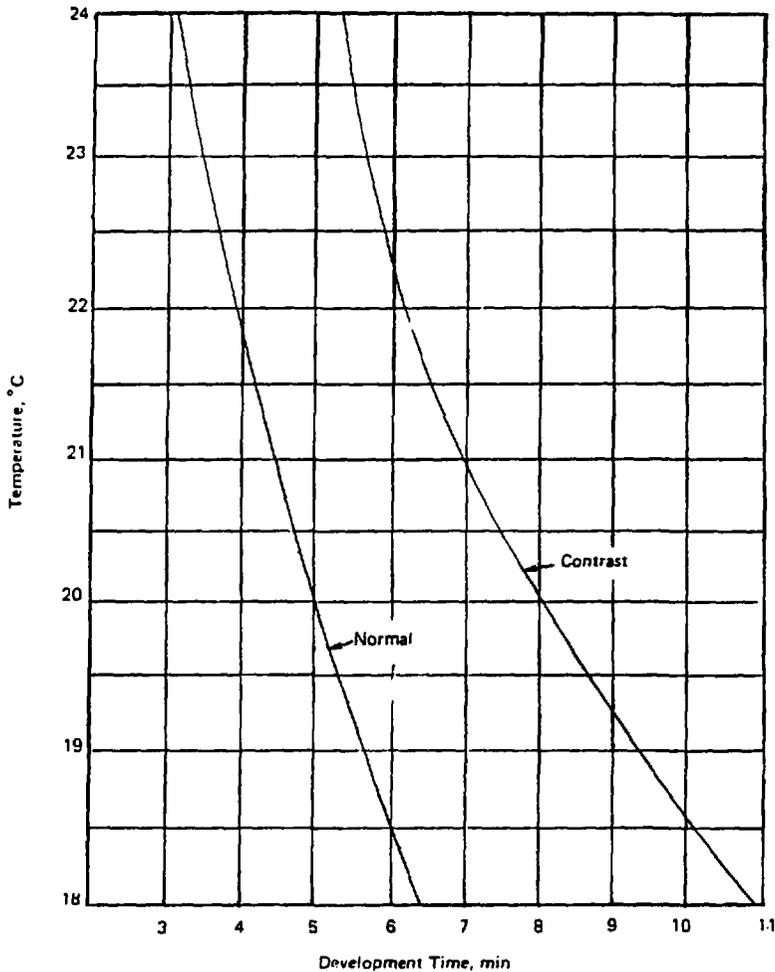
Figure 5.1 Time-temperature relationship for the development of a radiographic film.
