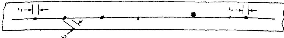
Sum of  $L_1$  to  $L_2$  shall be less than t in a length of 12t.
