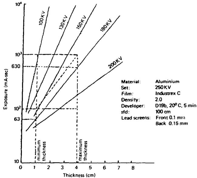
Figure 6.24 Diagonal method for determination of exposure.
