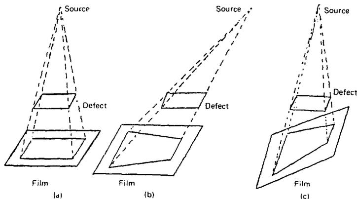
Figure 9.1 Effect of (a) normal beam, (b) oblique beam and (c) inclined film on the shadow.
