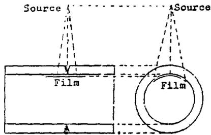
Figure 8.2. Film inside, source outside arrangement.
