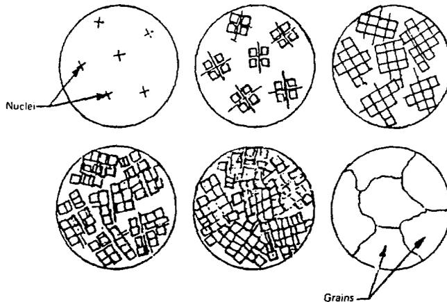
Figure 1.33 : Growth of crystals and grains during solidification.
