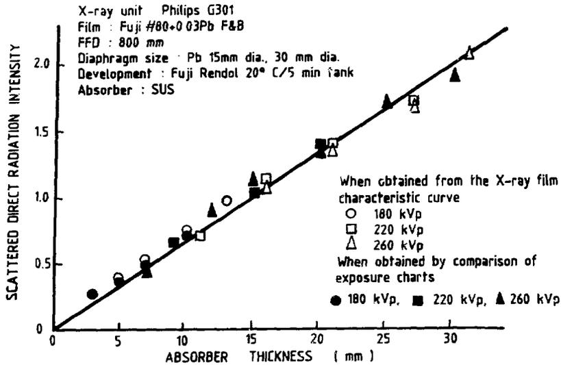
Figure 7.8 Relation between scattered direct radiation intensity and absorber thickness.
