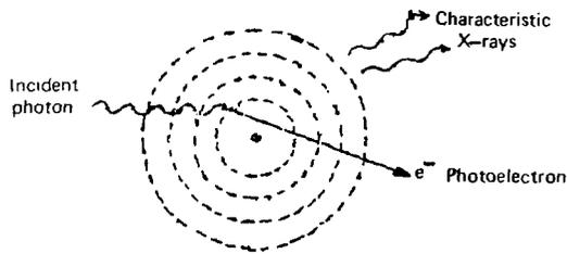
Figure 2.11 Photoelectric absorption
