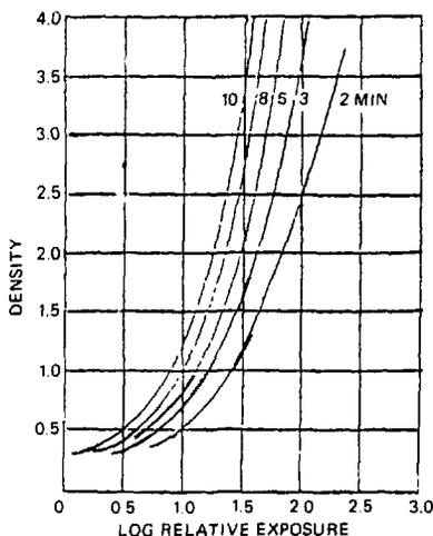
Figure 4.11. Characteristic curves of a typical industrial x-ray film, developed for 2,3,5,8 and 10 minutes.
