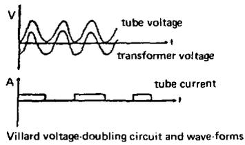
Figure 3.5. Villard voltage doubling circuit and wave forms
