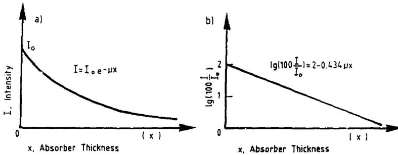
Figure 2.14 : Attenuation curve (a) in linear (b) in semilogarithmic scale
