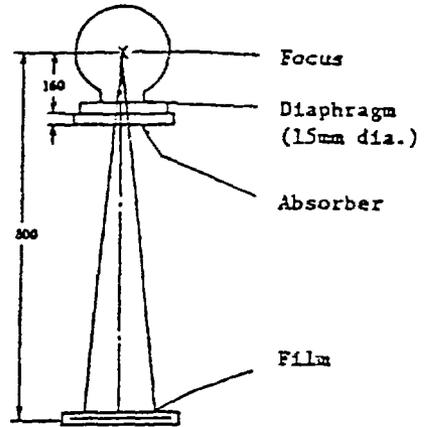
Figure 7.6 Radiographic arrangement
