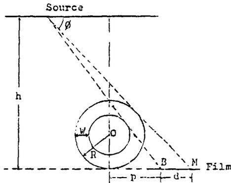
Figure 8.18 Wall thickness measurement of large diameter pipe.
