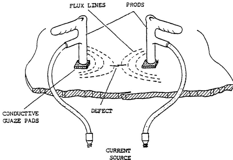
Figure. 1.8 : Magnetisation of irregular specimens.
