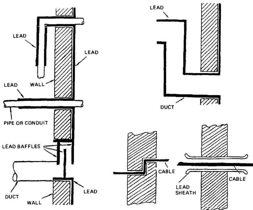
Figure 12.3 Methods of shielding when pipes, ducts, conduits or cables must pass through walls of exposure room.
