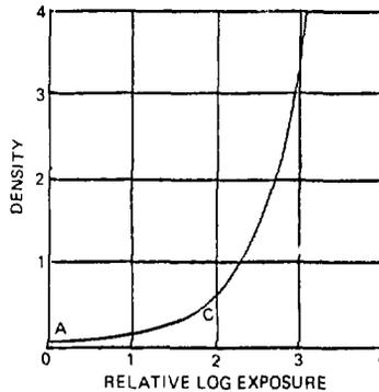
Figure 4.2 Characteristic curve of a typical direct-type X-ray film.
