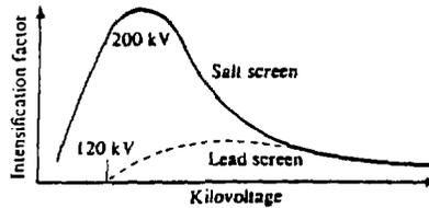
Figure 4.13 Variation of intensification factor with kilovoltage.
