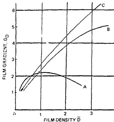
Figure 4.9 Film gradient against film density for various types of film. 'A' salt screen film used with salt screens. 'B' medium speed film used with metal screens or no screens. 'C' fine grain film used with metal screens or no screens.
