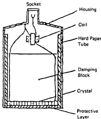
Figure 1.17 A typical normal beam single crystal ultrasonic probe
