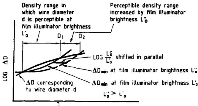
Figure 7.14 Relationship between density and penetrometer sensitivity (influence of film illuminator brightness)
