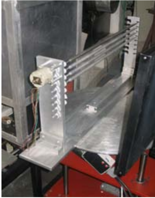
Fig. 56. Holder for nuclear fuel put on the sample holder.
