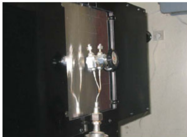
Fig. 61. The test object placed in front of the scintillator screen of the neutron imaging system with CCD camera.
