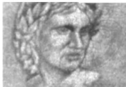
Fig. 77. NIER of a regular Brazilian bill showing one of the security marks.
