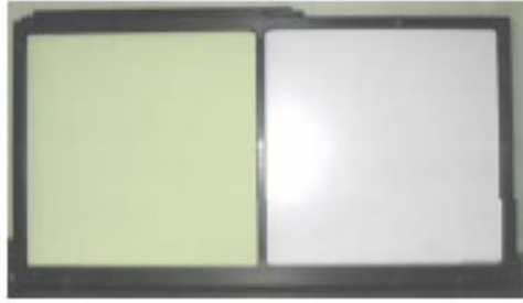
Fig. 44. The scintillator for neutrons (left) and the scintillator for gammas (right).
