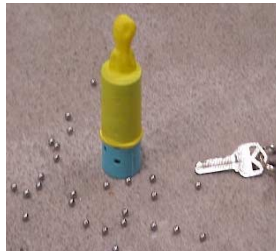
(b) Balloon Gun Impact Source with Ball Bearings
