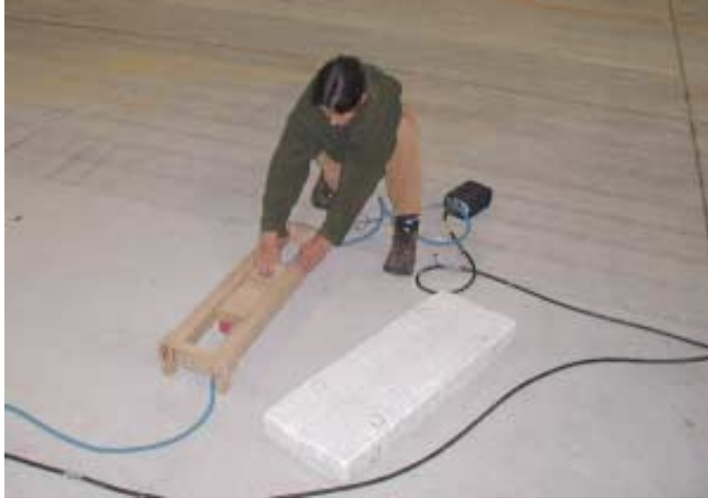
Figure 39 – CMP Concrete Thickness Measurements at the FAA Test Facility
