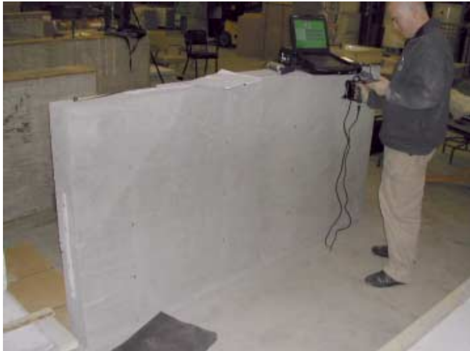
Figure 27 – Variable Thickness Concrete Slab During Testing
