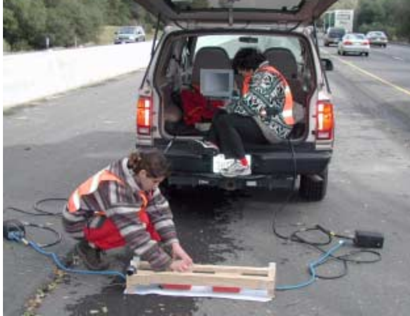
Figure 45 – CMP Data Collection at US 50 (note Teflon sheet)
