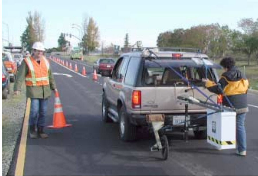
(a) Horn Antenna Data Collection in Right Wheel Path behind Lane Closure
