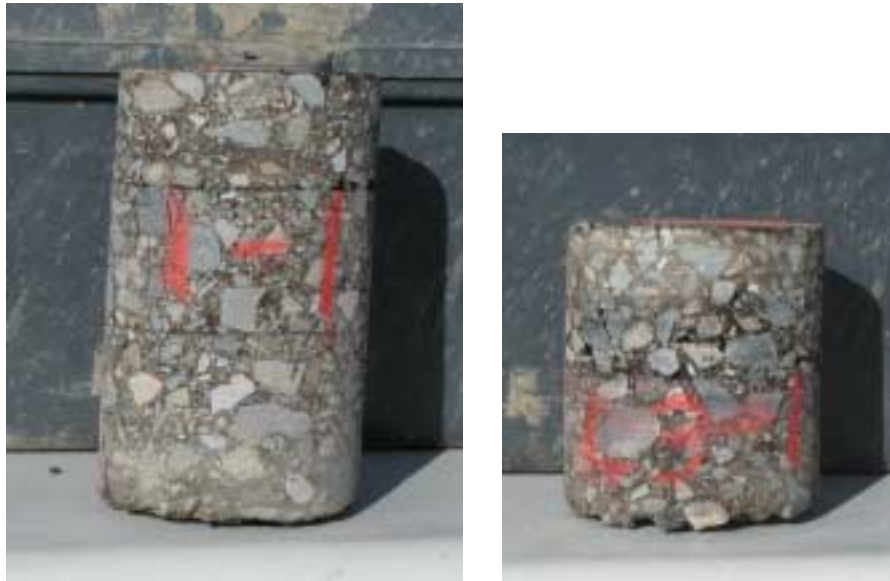
(a) Inside Lane, 163 mm (6.5") (b) Outside Lane, 100 mm (4")
