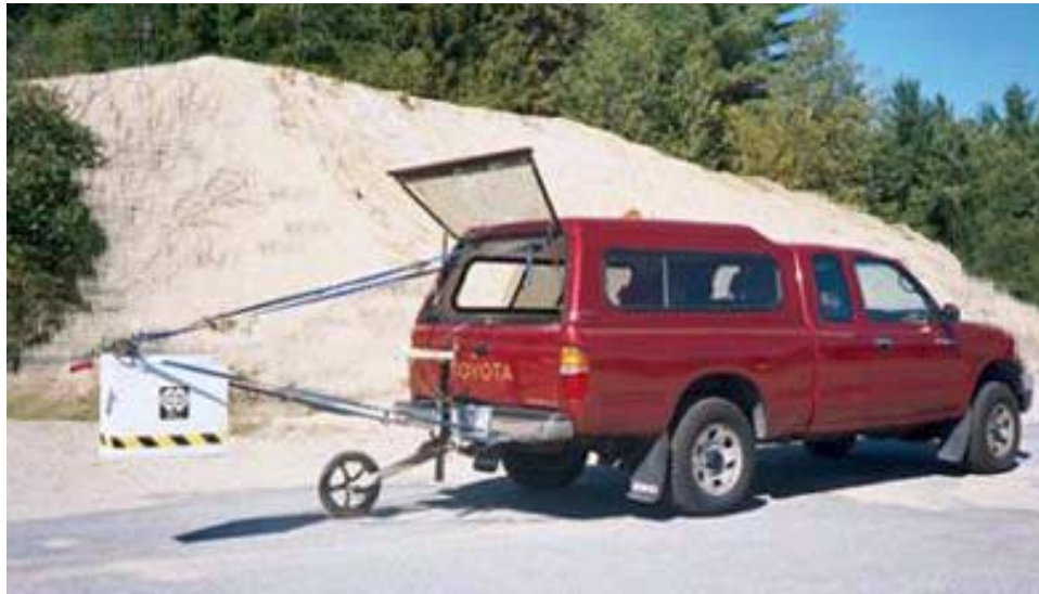
Figure 30 – Horn Antenna Equipment Setup
