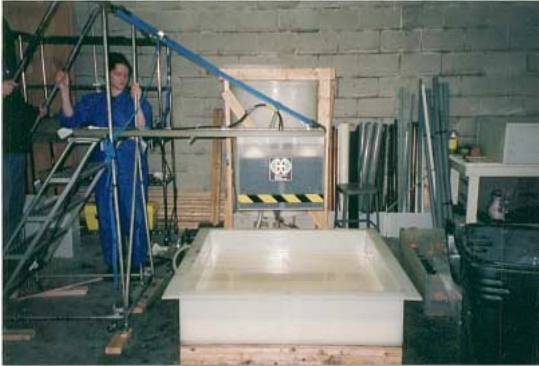
Figure 18 – Data Collection Over the Emulsion Using the Model 4108 Horn Antenna
