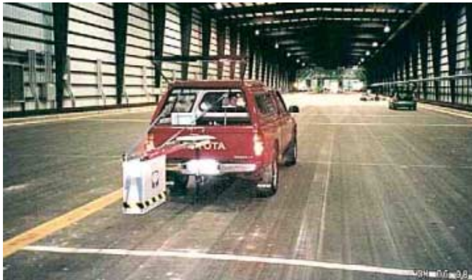
Figure 33 – Horn Antenna Data Collection Setup at the FAATC
