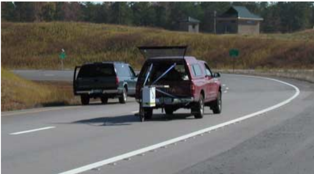
Figure 38 – Horn Antenna Data Collection at the NCAT Facility in Auburn, AL
