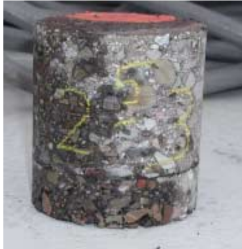
Figure 48 – Sample Core from I-5 Showing AC Layers
