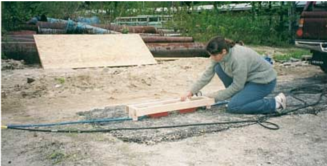
(b) Using Ground-Coupled Antennas with CMP Method
