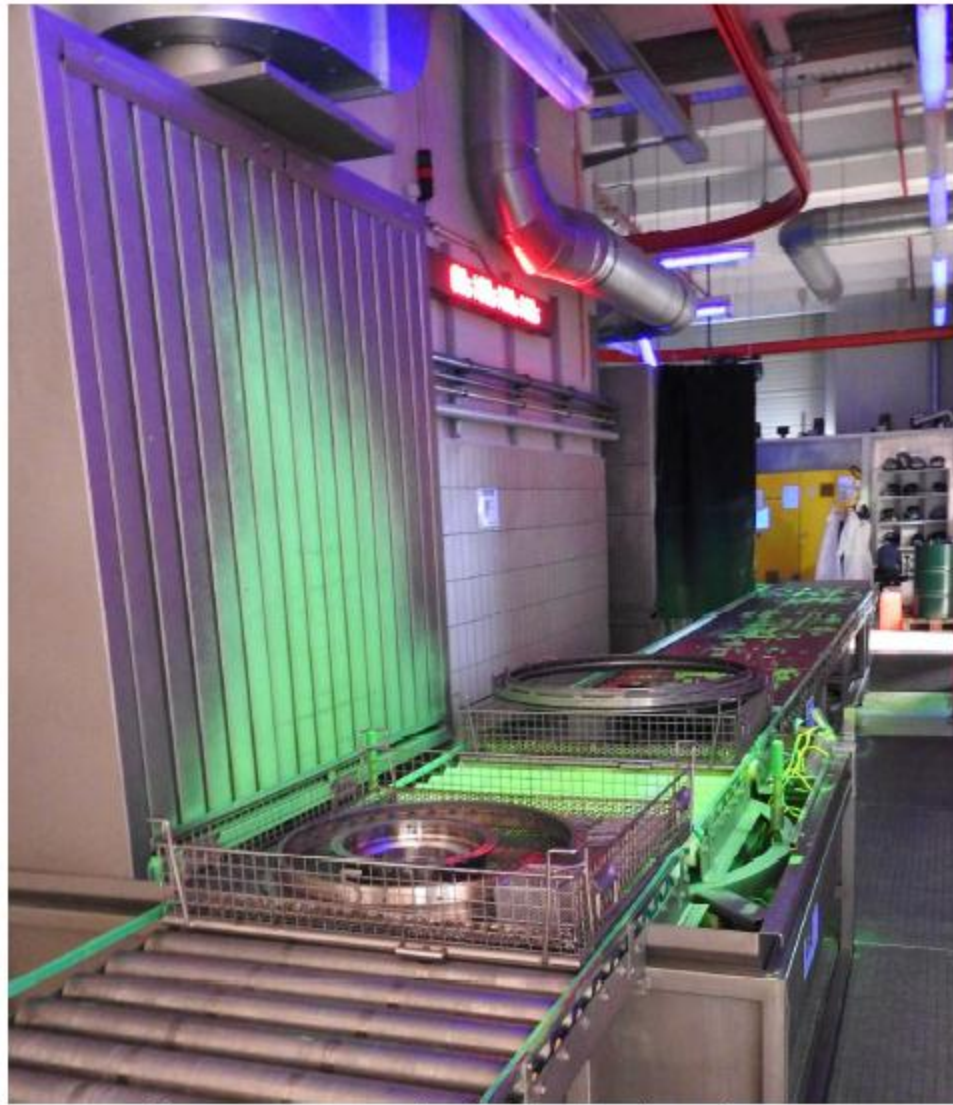
Penetrant test processing line for turbo-jet engine components
