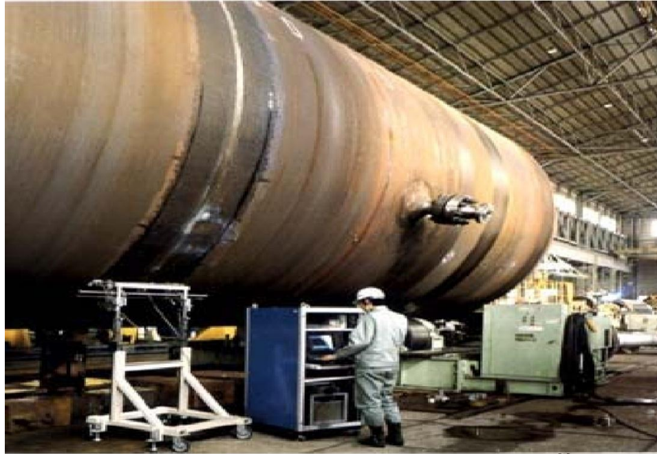
Fig. 8 TOFD being done for a heavy walled pressure vessel at shop [5]
