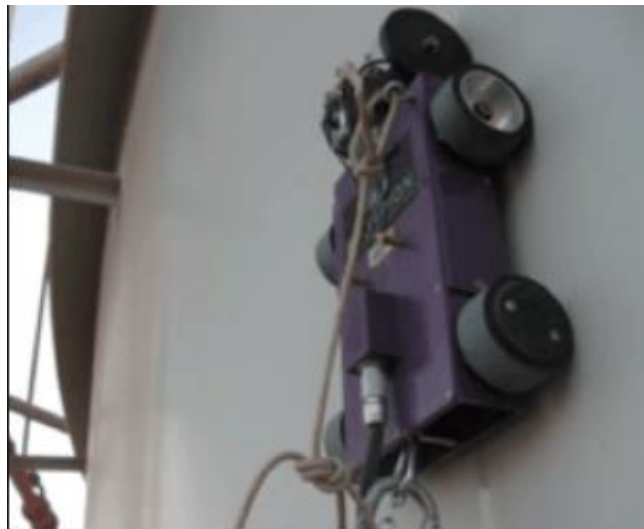
Figure 2. 4 Wall climbing robot in-service inspection (ENVIROPRO, 2018).
