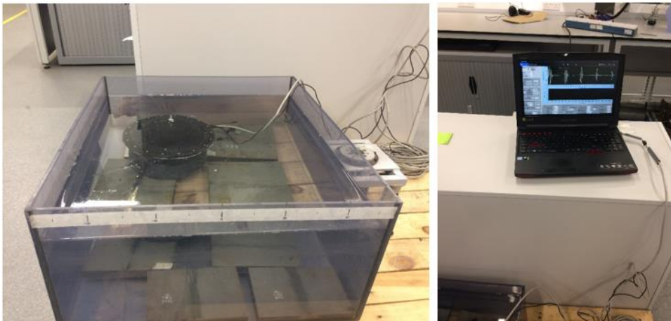
Figure 4. 15: NDTBOT in water tank inspection
