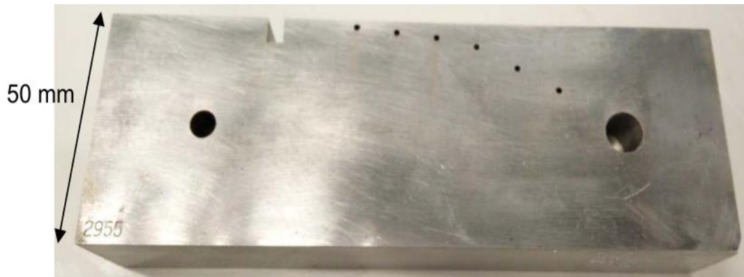
Figure 4. 12: Steel calibration block with a thickness of 25 mm
