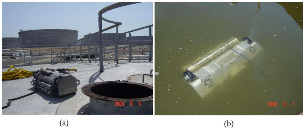
Figure 2. 5: in-service inspection robot RobTank (2003).
