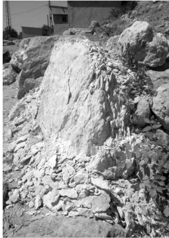
Figure 6.2 Catastrophic decay of limestone (probably Gaziantep formation) in figure 40 in 2012 (Photo© Engelbert Winter 2011).
