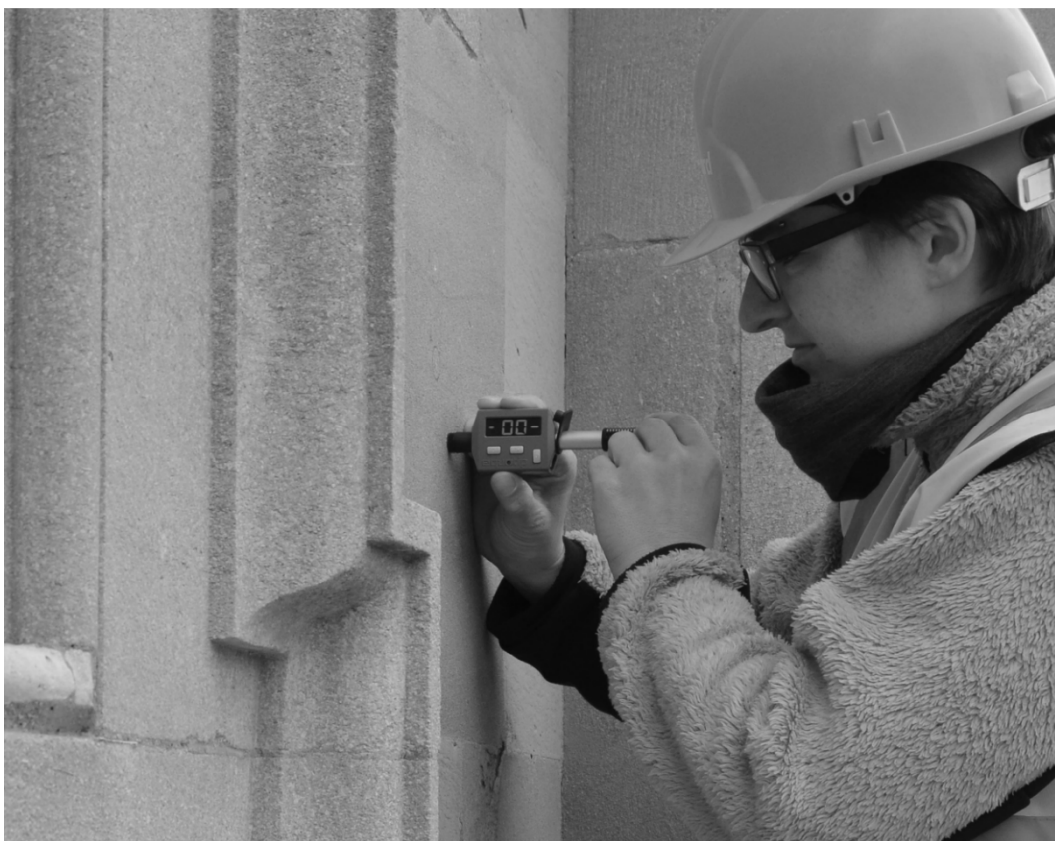
Figure 4.1. Equotip Piccolo 2 with impact body D on-site at Radcliffe Camera, Oxford.
