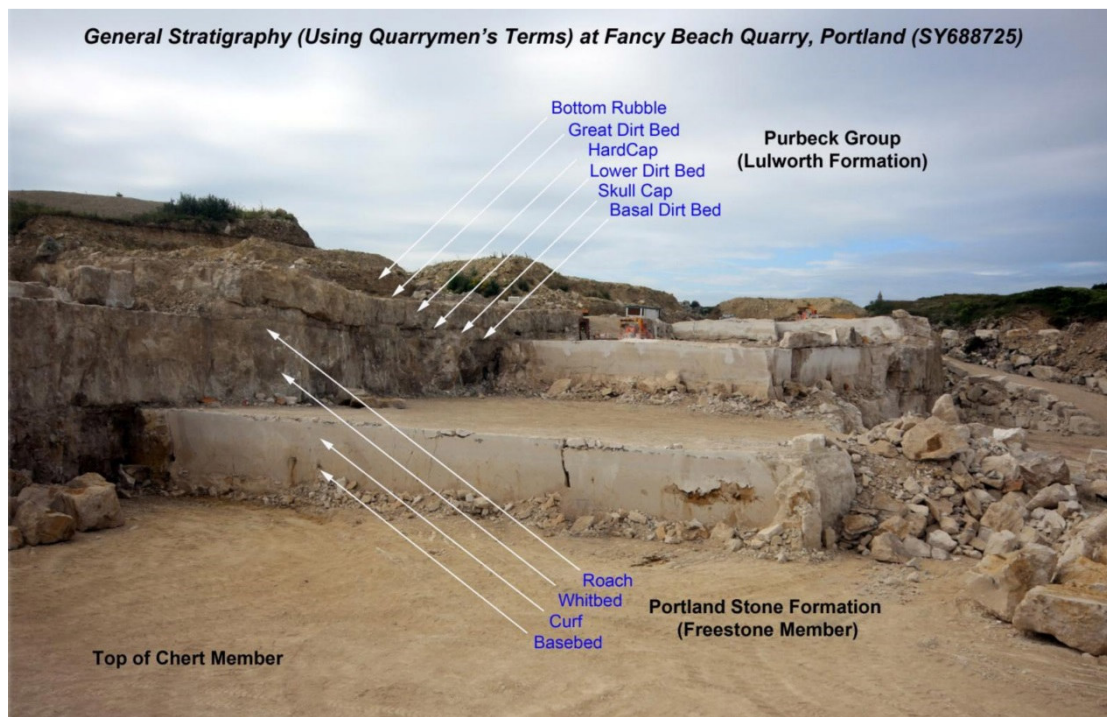
Figure 2.3 Portland limestone beds, general stratigraphy (using quarrymen's terms) at Fancy Beach Quarry, Portland (UK, SY688725; source: Godden, 2012, p.8)
