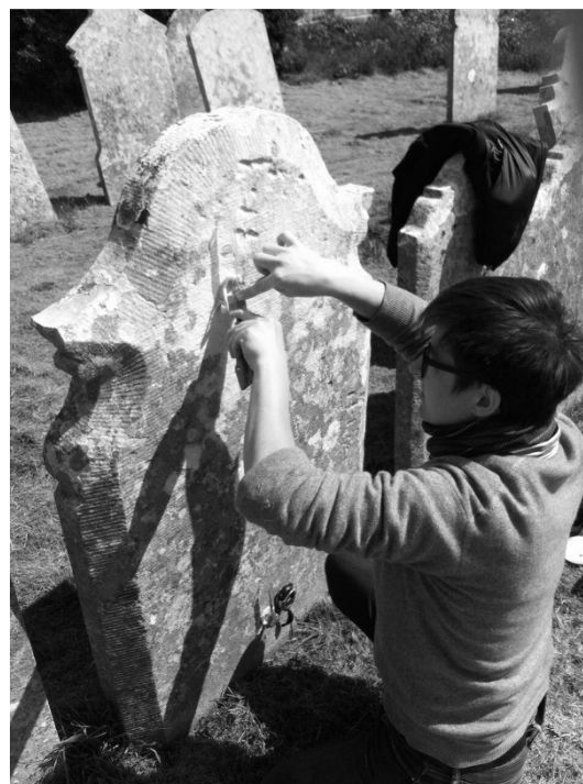
Figure 2.14 In situ application of Karsten tube to a limestone headstone during field work at St George's Church cemetery in Portland, Isle of Portland (UK)
